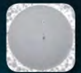
Mated 5x dirty then cleaned results in severe permanent damage
